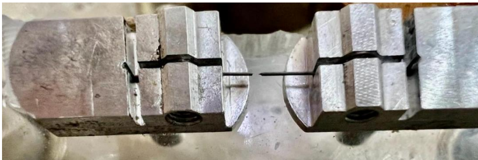
Figure 1. shows the technique used for the fabrication of the overhanging electrodes.
